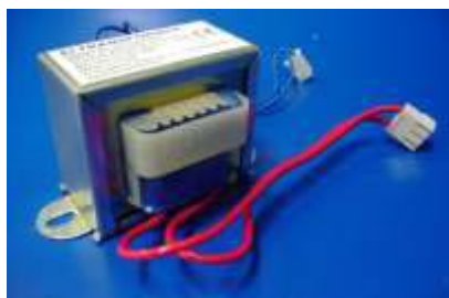
Transformador 127VAC 24V-700mA-(070378) 220VAC 36V-800mA- (070379)
